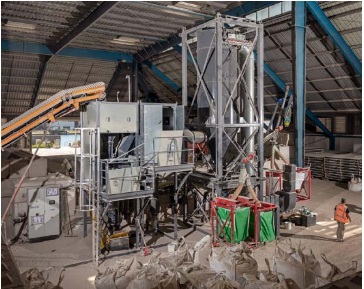
Concrete recycling at New Horizon involves a “smart refiner” that separates the finest particles — cement dust and sand. Max Pinckers for The New York Times
