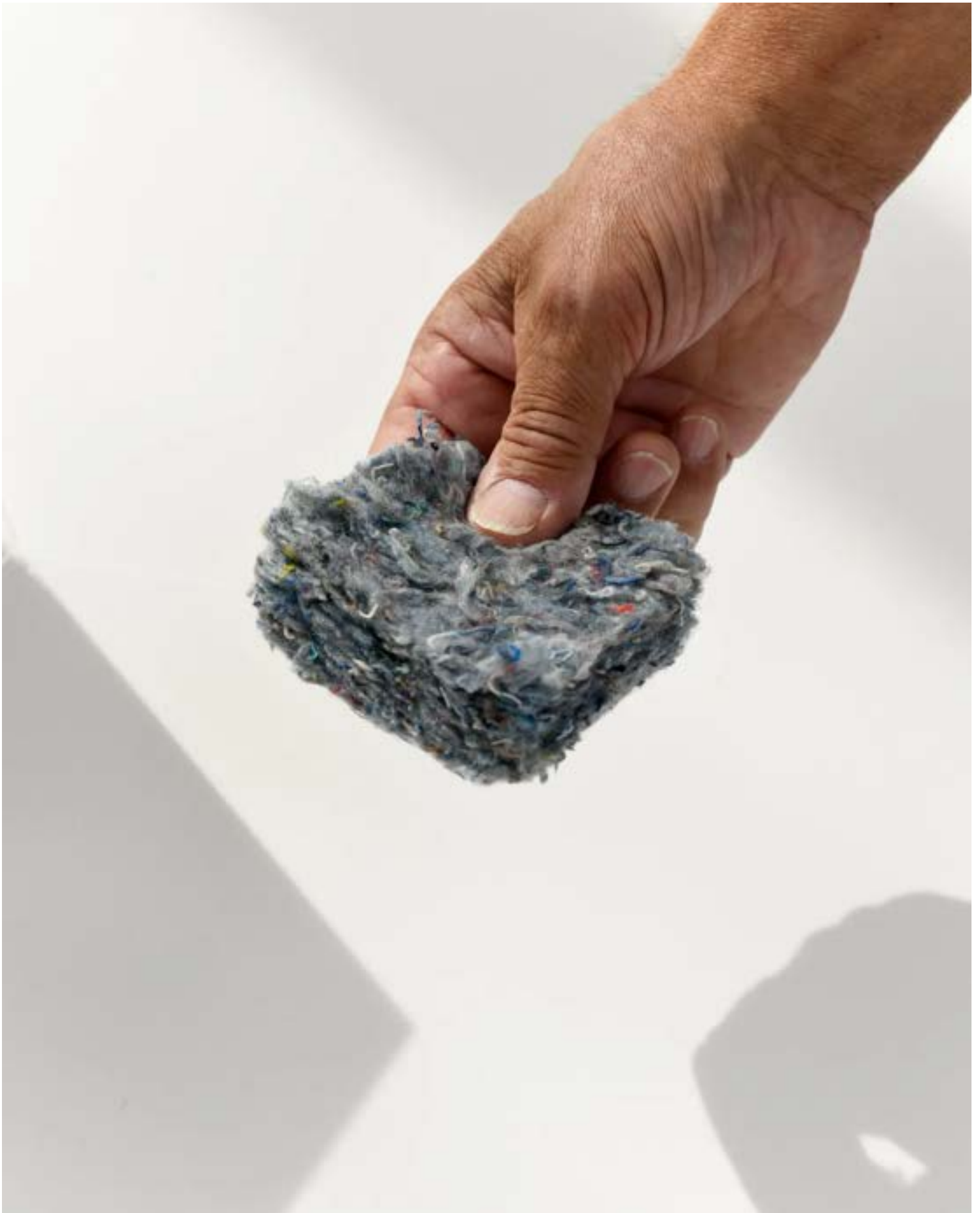
Discarded clothing is turned into insulation in one of the building's Thomas Rau designed. Max Pinckers for The New York Times
